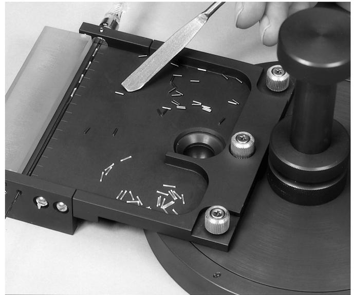
The Seed Slider connected to the Seed Sterilization and Sorting Tray.
