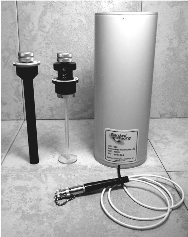
This test tool, intended to detect x-ray contamination in your source, is made with a 7 mm plastic wall thickness. This specific wall thickness will absorb essentially all of the beta radiation, while allowing the bremsstrahlung radiation to pass through the source holder for measurement.
