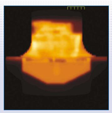
Examine the fluence dose image of a film placed between acrylic slabs of the IMRT Phantom.
