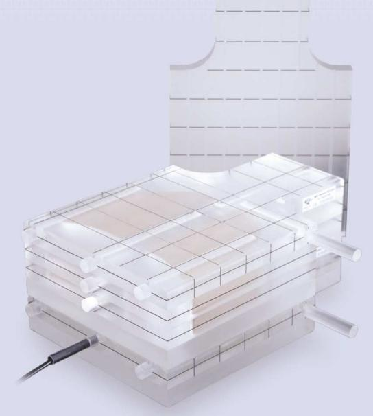
Simultaneous acquisition of absolute, relative and point dose measurements.
