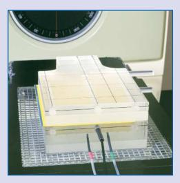
Phantom on accelerator treatment couch ready for treatment.
