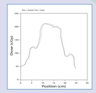
Analysis of a horizontal fluence dose profile of the measured film versus the calculated dose on the RTP.
