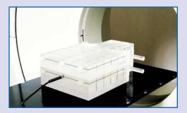
Phantom positioned on the simulator couch ready to be scanned.
