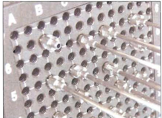
A close-up shows the Needle Collets threaded into the Needle Channels of the Template; some with inserted Rigid Metal Needles and some without.
